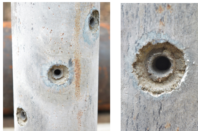
The EchoFrac shaped charges in the DS Echo gun system maintain cement integrity between inner and outer casing while creating uniform EHD and consistent AOF.
