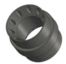
In addition to preventing inadvertent contact, this unique model ensures minimal velocity reduction of the drop bar as it passes through the insert, as the ports provide additional flow channels for fluid displacement by the bar as it travels downward.
